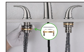
2.Put rubber gasket, steel washer and the nut in sequence upward. Screw the nut in clockwise and tighten. Then use a screwdriver to fully tighten the locking screw on the nut.
